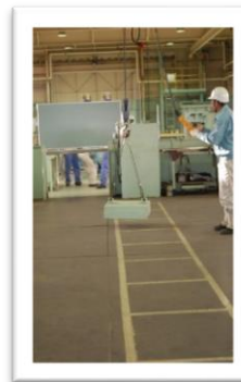
Swinging of hoisted load danger
